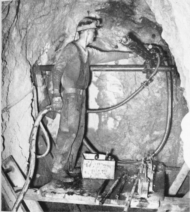
A miner, way down in his stony burrow with a high compression drill, cuts away at a seam of rock which bears the copper ore. He hustles out the "goods" to feed the Scovill Casting Shop.
